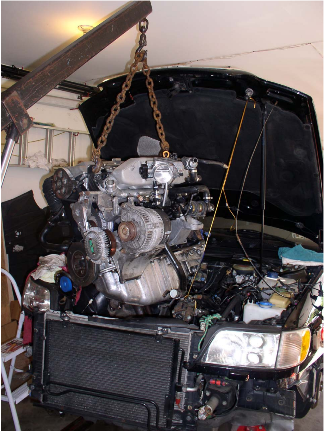
10. Engine on hoist (before shortening chain):
